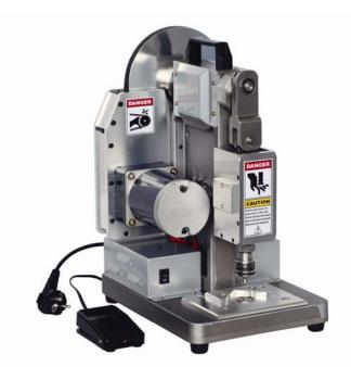
The **Model MP10** is an innovative mini-press designed for grommet applications. Pre-punched work is not required as the power of the MP10 coupled with self-piercing grommets consistently delivers good settings. Presently the MP10 is available for 8mm and 12mm grommets. This machine is built on a cast frame and designed for safe operation, portability and ease of use.
