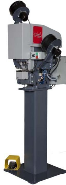
(Shown on Standard Pedestal Base with Barrier Guarding Removed)
